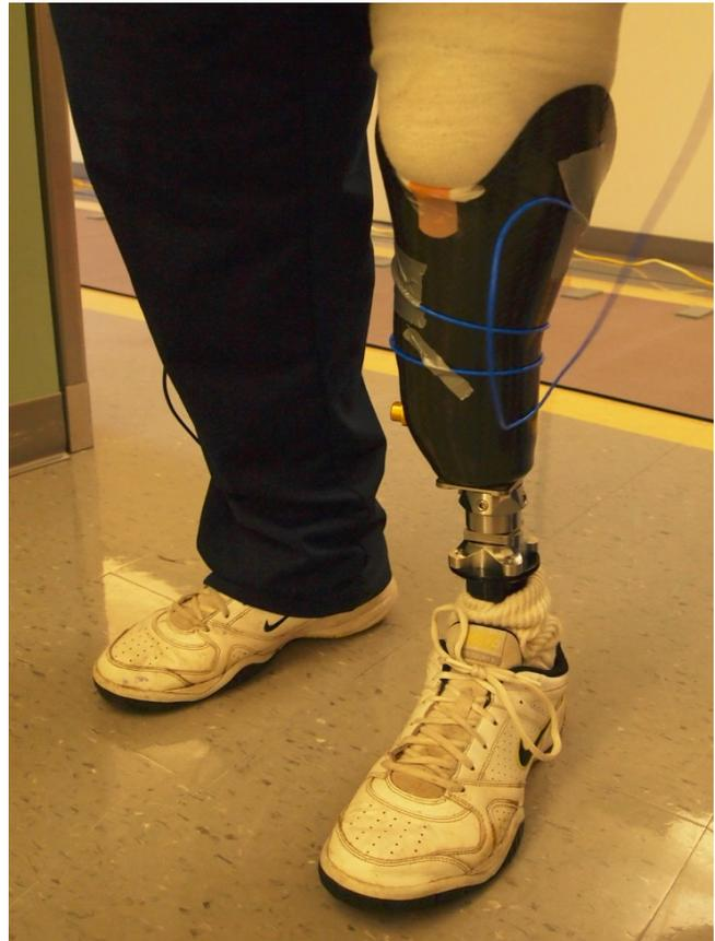
**Figure 1: The kinetic sensor attached to a subject's prosthesis**
